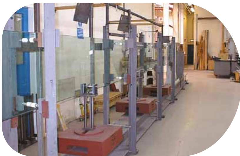
Glass Fin testing, Pilkington R&D Centre, UK.
